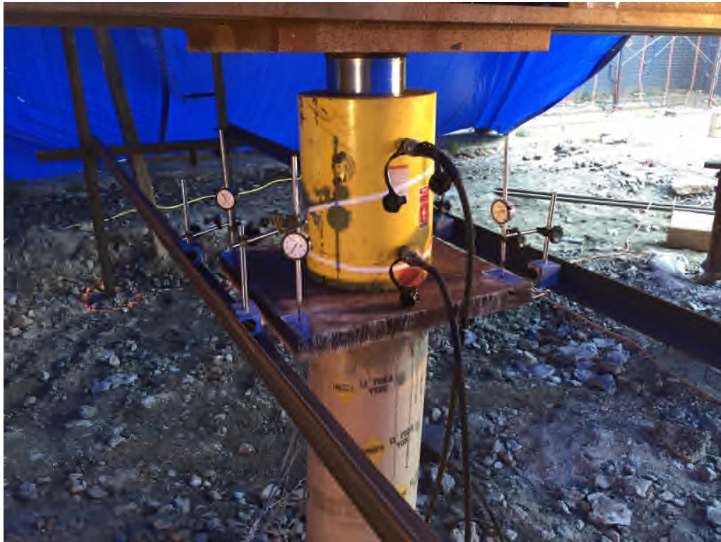
Photo 2: Typical Jack and Dial Gauge Measurement Setup
